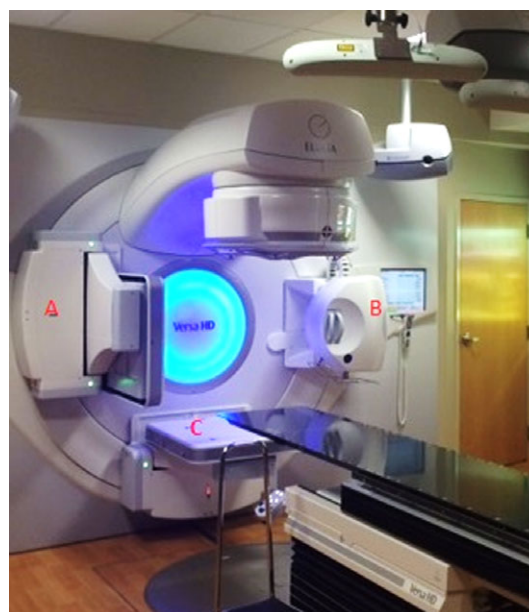
FIG. 1. The X-ray volume imaging (XVI) guidance system and iViewGT image system of the Elekta VersaHD radiation delivery system are shown. (a) a-Si flat panel detector of the XVI, (b) kV X-ray source of the XVI and (c) iViewGT imaging panel.
