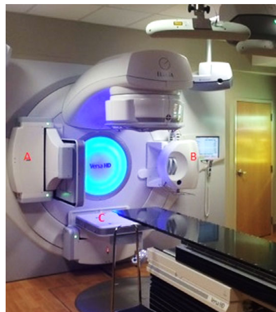
FIG. 1. The X-ray volume imaging (XVI) guidance system and iViewGT image system of the Elekta VersaHD radiation delivery system are shown. (a) a-Si flat panel detector of the XVI, (b) kV X-ray source of the XVI and (c) iViewGT imaging panel.
